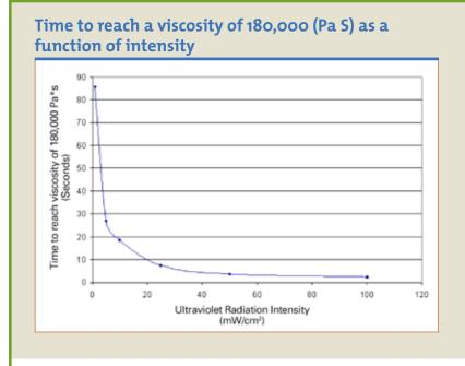
optic coating sample exposed to UV radiation from a programmable UV LED source. An intensity of 1.0 mW/cm<sup>2</sup> showed poor cure characteristics when compared to intensities of 5.0 mW/cm<sup>2</sup> and higher. Also, there was no significant difference between 50.0 and 100.0 mW/cm<sup>2</sup>, suggesting 50.0 mW/cm<sup>2</sup> is the optimum UV curing intensity for this material.
