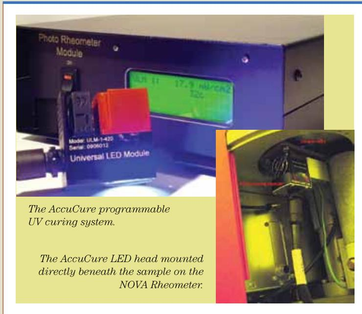
The AccuCure programmable UV curing system.
