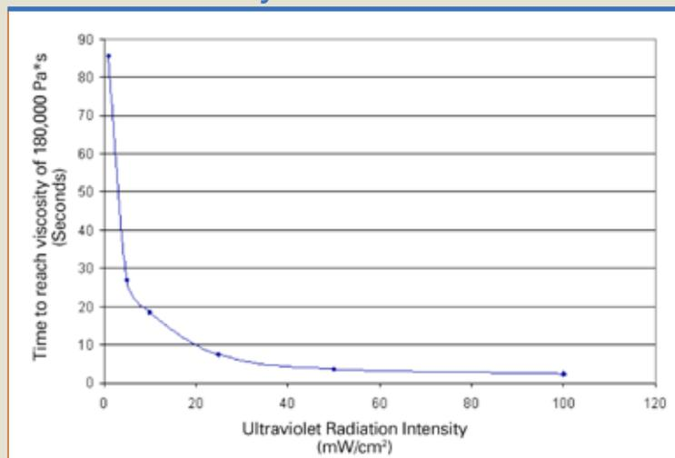
optic coating sample exposed to UV radiation from a programmable UV LED source. An intensity of 1.0 mW/cm<sup>2</sup> showed poor cure characteristics when compared to intensities of 5.0 mW/cm<sup>2</sup> and higher. Also, there was no significant difference between 50.0 and 100.0 mW/cm<sup>2</sup>, suggesting 50.0 mW/cm<sup>2</sup> is the optimum UV curing intensity for this material. ▀
